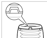
FIG. 15 Hold the housing with the opening upwards and insert the folding balloon. Check the correct seat of the folding balloon.
